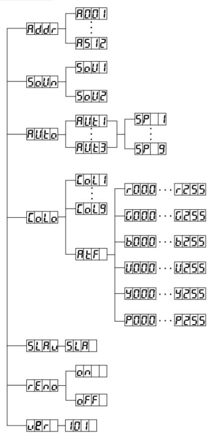
Addr - DMX Address Setting via control board
