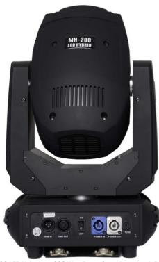
The MH-200 LED Hybrid is a 200 Watt Beam/Spot Movinghead. By means of an extra lens the beam can switch between a beam angle of 5 or 13 degrees. With this you can not only make tight beams, but also project beautiful gobos. The MH-200 LED Hybrid also has 6 rotating gobos, 8 static gobos and 7 colors. Finally, there is also a 3 facet rotating prism to make it complete!
